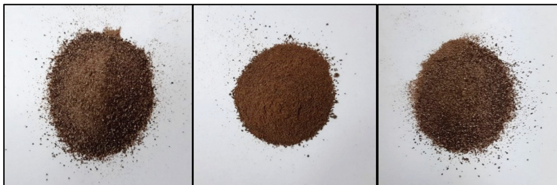
Figure 1. Pectin samples extracted from 'Saba' banana peels using various extraction methods. (L-R: acid-extracted, enzyme-extracted, microwave-assisted extracted pectin)
